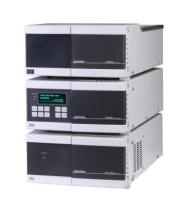
System contains manual injector and **ECOMAC** software which include drivers for all ECOM units.
