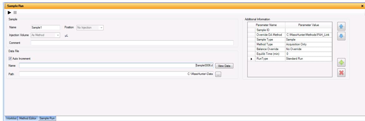
You can run a Data Analysis method from this window by selecting **Both Acquisition and DA or DA Only** for the **Method Type**. In addition, you have to set **Override DA method** to indicate which Data Acquisition method contains the DA (Data Analysis) method to execute. You always have to do this.
