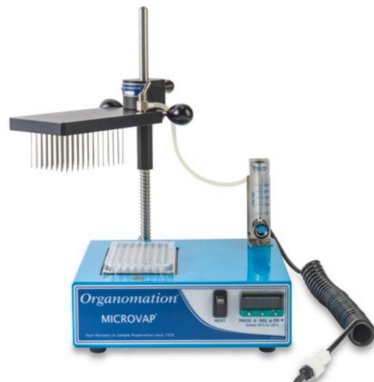
phase extraction cartridge elutions. Alternatively, the single position microplate configuration is ideal for low-volume applications, such as organic solvent removal from HPLC fractions.
