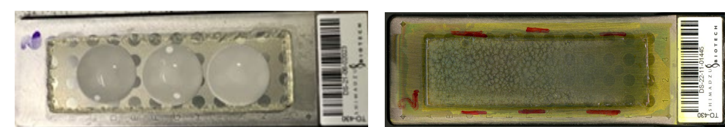
Figure 2 Sample preparation for exo-metabolite analysis on Fleximass-DS MALDI target slides
