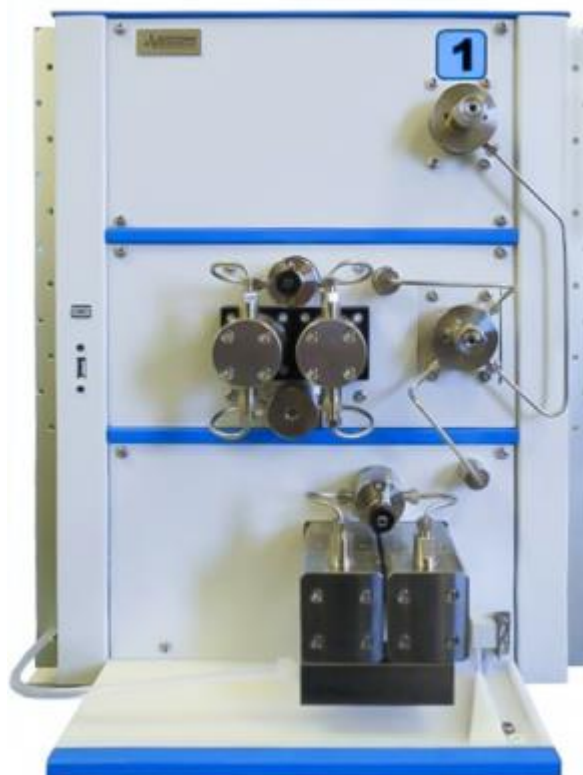
FRONT VIEW UNIT WITH ASCENDING / DESCENDING VALVE
