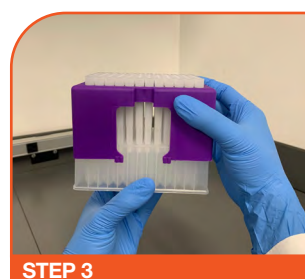
STEP 3 Remove 96-Autorack containing Mitra devices from the collection plate and discard
