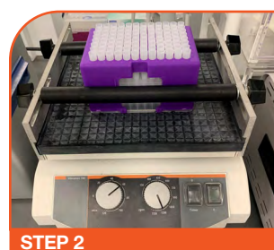
STEP 2 Shake collection plate and 96-Autorack assembly on Vibramax 100 (Heidolph) for 1 hour @ 1200 rpm
