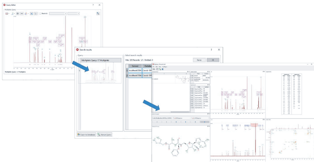
Figure 4 – A spectral search matching all the multiplets in a spectrum to find previous examples of this compound
