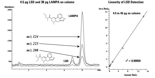
Conditions: Instrument: Agilent 1100 LC/MSD System Column: ZORBAX Eclipse XDB-C8, 2.1 x 50 mm, 5 $\mu$ m, Agilent P/N: 960967-906 Mobile Phase: 15 : 85, ACN : H<sub>2</sub>O containing 10 mM ammonium formate, pH 3.7 F=0.3 mL/min, Inj vol: 30  $\mu$ l, Temp: 30°C, Det. MS HP 1100 MSD Conditions: SIM mode, Ions: 324.2, 223.1, 208.1 Fragmentor (dynamically ramped) 100V at 324.2, 148V at 223.1, 170V at 208.1
