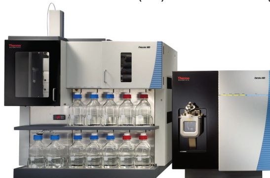
FIGURE 5. Prelude MD HPLC (Left) and Endura MD MS (Right)
