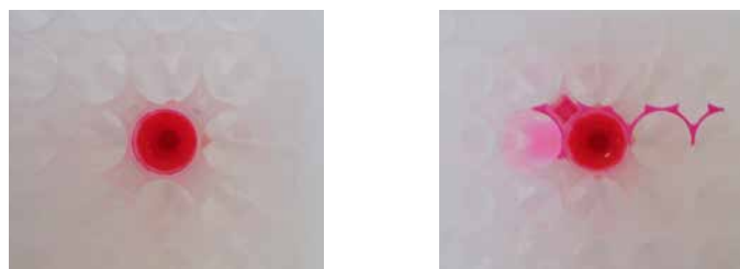
Figure 5c. 1.7 and 1.8 mL volumes mixed in a 2 mL/well nominal volume round collection plate (Vortex Genie, setting 3) showing potential cross contamination when max fill volume is exceeded.
