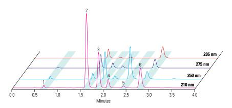
Figure 5. Up to four wavelengths can be recorded simultaneously with up to 5 Hz data collection rate, making the four-channel mode compatible with even fast chromatography.
