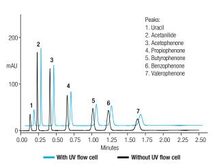
Figure 9. Overlay of two isocratic UV chromatograms, one obtained with the 45 nL UV monitor before the detecting cell (blue), one without (black). The plate count of all peaks remains constant.
