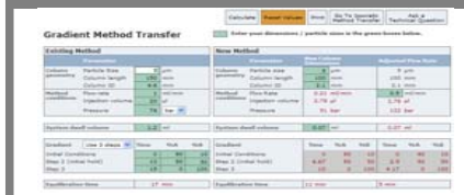
FIGURE 4. Gradient method transfer calculator ( http://www.hplctransfer.com/ ). Transfer of gradient method to a shorter column (from 150 x 4.6 mm to a 100 x 2.1 mm).
