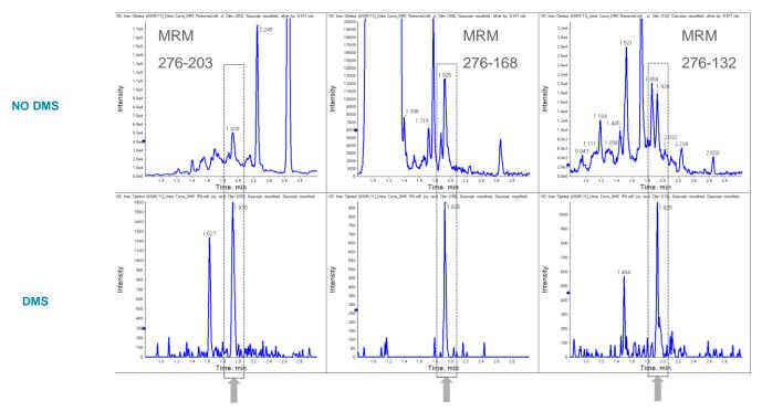
Figure 3. Analysis of Clenbuterol in Urine. This assay suffers from matrix interferences in all three MRM channels (top). Using SelexION Technology with isopropanol as a chemical modifier resulted in the reduction or elimination of interferences in all three MRM channels (bottom).
