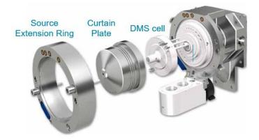
Figure 1. SelexION® Technology. The DMS interface is directly coupled to the orifice plate. A modified curtain plate accommodates the DMS cell which can be easily installed and removed without the use of any tools and without venting the system. The source extension ring enables use of the standard SCIEX sources.
