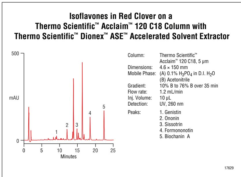
Red clover is rich in isoflavones that may have useful pharmaceutical properties. Dionex ASE Accelerated Solvent Extractor system is a convenient, automated process that uses heat and pressure in a closed cell to extract samples with reduced time and solvent consumption. The high resolution of the Acclaim C18 column gives a clean separation even with this complex sample matrix.
