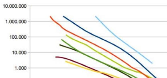
GPC-calibration curves AppliChrom ABOA StyDiViBe 300 x 8 mm, THF, 1 ml/min, PMMA standards, M[da] vs.  $V_e$  [ml], porosities: 35A, 100A, 500A, 10<sup>3</sup>A, 1500A-BPT, 10<sup>5</sup> A-BPT, 10<sup>6</sup> A-BPT, 10<sup>7</sup> A-BPT
