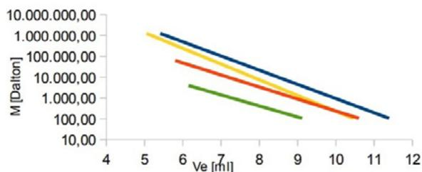
Measurement ranges for AppliChrom ABOA SuperOH GPC/SEC columns, 300 x 8 mm, measured in water using PEG/PEO-standards: Porosities **100, 200, 300, 400**
