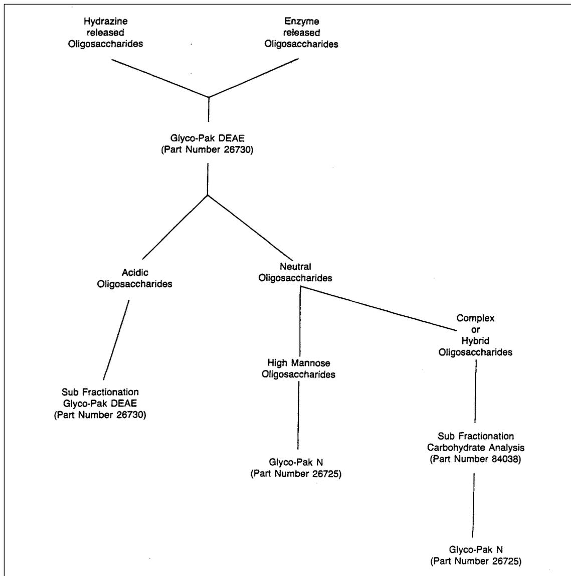
Oligosaccharides released by hydrazinolysis or enzyme treatment may be simultaneously separated into neutral and multiple acidic fractions (depending on the number of sialic acids or degree of sulfation) on the Glyco-Pak DEAE column (P/N 26730). Acidic fractions may be further purified on the Glyco-Pak DEAE by changing the mobile phase and/or gradient conditions.
