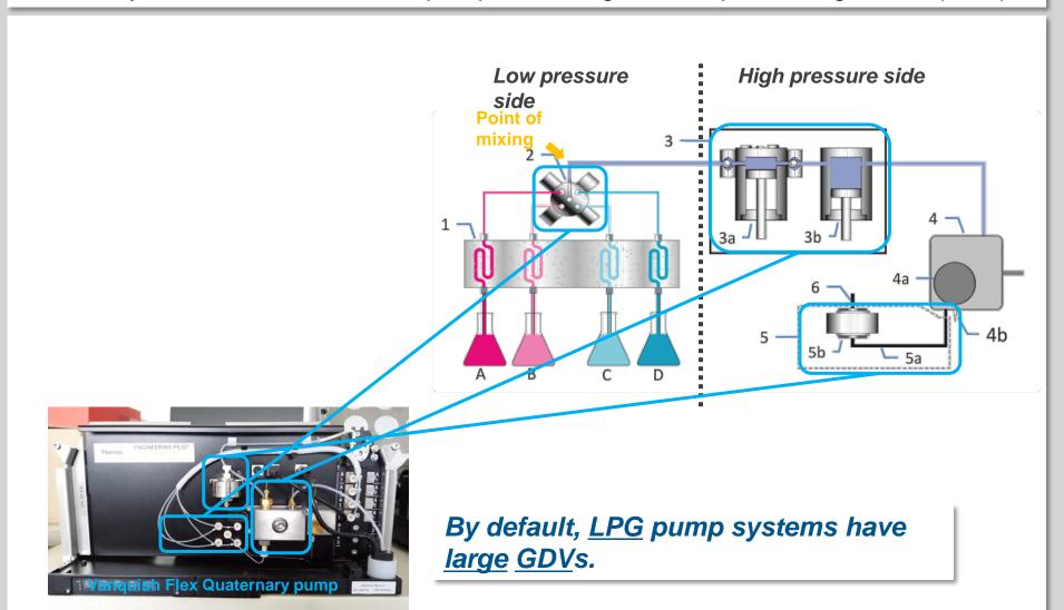
UHPLC systems can use different pump technologies: Low pressure gradient (LPG)
