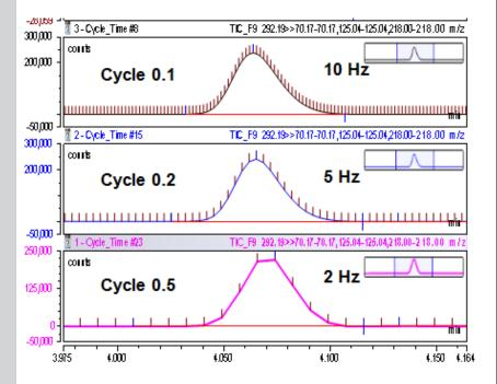
At least 10 Hz are required to obtain RT SD = 0.001 min for peak width at 50% of 0.025 min (1.5 s).
