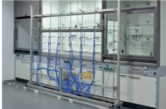
EN 14175-6 type tested fume hood control in acc. with 5.4 Measuring in the outer measuring level
