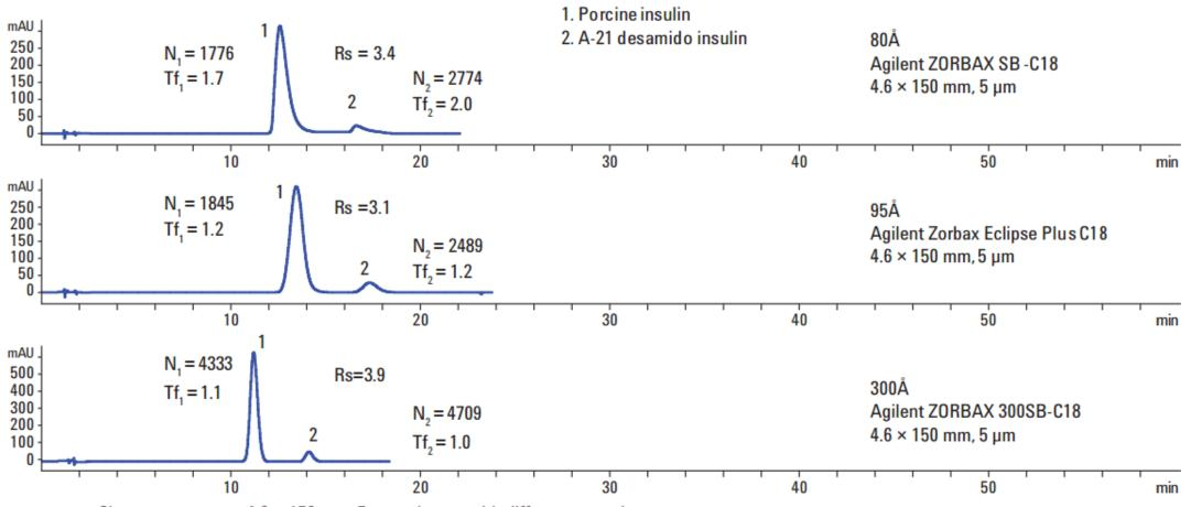
Chromatograms on  $4.6 \times 150$  mm, 5  $\mu$ m columns with different pore size.
