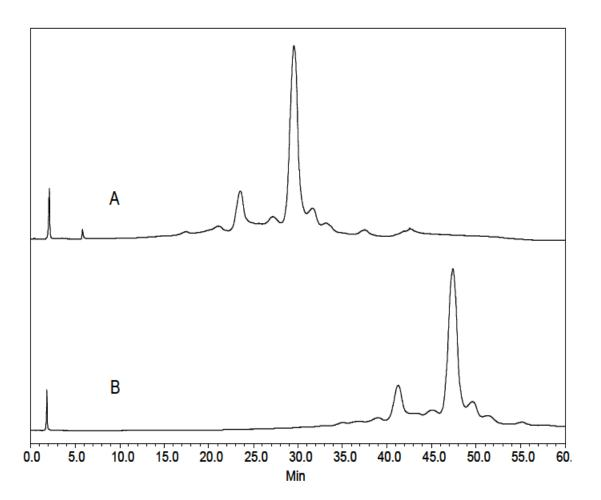
Column: Agilent Bio MAb, NP10, 4.6 x 250 mm Mobile phase: A: 10 mM phosphate; B: A + 0.1 M NaCl pH: A = pH 7.5B = pH 7.0Gradient: 15–65%B in 60 min Flow rate: 0.8 mL/min Sample: Monoclonal Antibody Injection: 10  $\mu$ L (1.5 mg/mL) Temperature: 25 °C Detection: UV 214 nm
