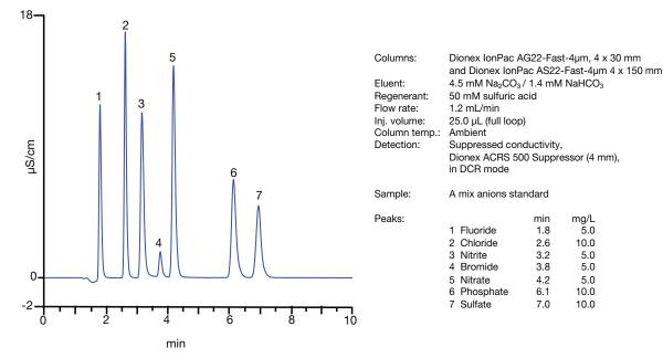
Figure 2. Separation of inorganic anions using the Dionex IonPac AS22-Fast-4µm column.
