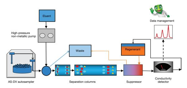
Figure 1. Illustration of an IC system in DCR mode.
