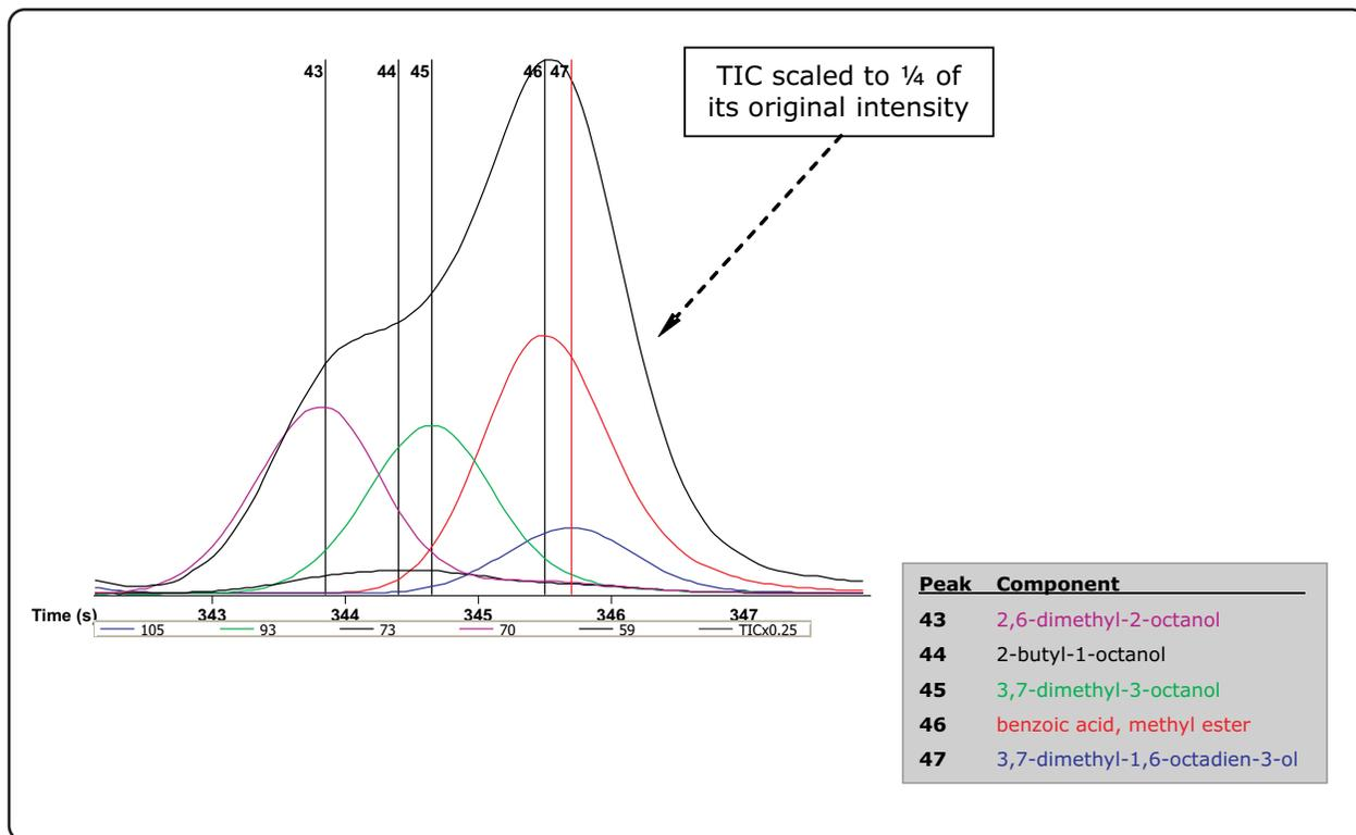
**A segment of the TD-GC-TOFMS chromatogram where five peaks coelute. True Signal Deconvolution® (TSD) provides the ability to detect all five of the coeluting peaks while providing an accurate identification of each peak.**
