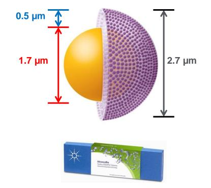
Ready to use AdvanceBio AAA kit (standards and reagents) All Agilent LC systems, including Infinity II systems AdvanceBio AAA columns Poroshell particles Fast and rugged
