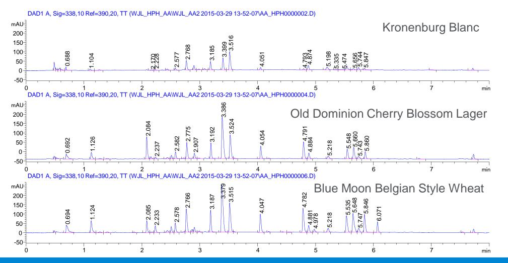
Quantity and diversity of amino acids is evident. Can be used to monitor and compare batches.
