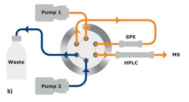
Figure 2. Switching Valve Configuration a) (Top) Valve position 1–2; b) (Bottom) Valve position1–36
