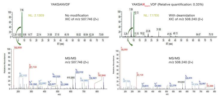
Figure 6. High-quality MS/MS data enables confident identification of low abundant deamidated peptide and relative quantification of the deamidated peptide vs. non-deamidated peptide using the integrated peak areas of the precursor ions.
