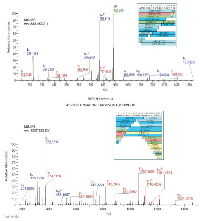
Figure 3 continued. N-terminus sequences of AAV6 VP1, VP2, and VP3 proteins were confidently identified with high-quality MS/MS data.
