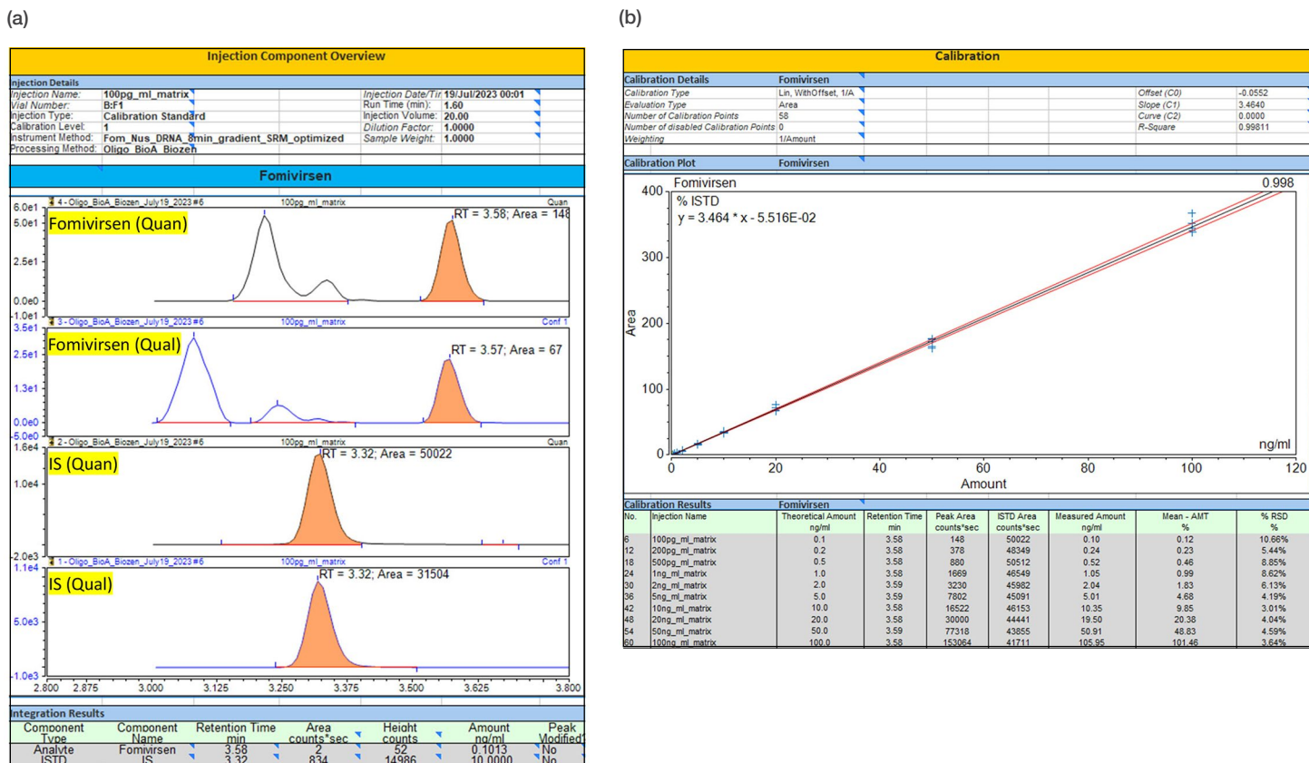
Figure 4. Example of a summary report for the quantitation of fomivirsen generated by Chromeleon CDS. (a) Sample injection information and integrated peak details, (b) calibration plot and the results for each calibration level (n=5)
