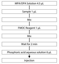
Fig. 1 Derivatization Flow with the Automatic Pretreatment Function
