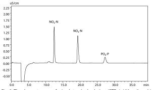
Fig. 2 The chromatogram of mixed standard solution (STD 4: 100  $\mu\text{g/L}$  each)
