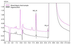
0.0 2.5 5.0 7.5 10.0 12.5 15.0 17.5 20.0 22.5 25.0 27.5 30.0 32.5 35.0 37.5 min Fig. 4 The chromatogram of digestion blank and mixed digest-check sample (Diluted 30 times after digestion)
