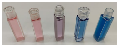
Fig. 8 Cobalt Chloride Solutions (60 °C) Pure water to acetone solvent ratios from left to right: 1:1, 1:2, 1:3, 1:4, and 1:5
