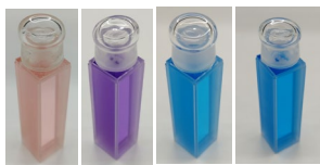
Fig. 4 Cobalt Chloride Solutions (50 °C) Solvents from left to right: pure water, methanol, ethanol, and acetone
