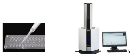
Fig. 3 Left: Applying Samples and Matrix Solutions to MALDI Plate Right: MALDI-8030 Benchtop MALDI-TOF Mass Spectrometer
