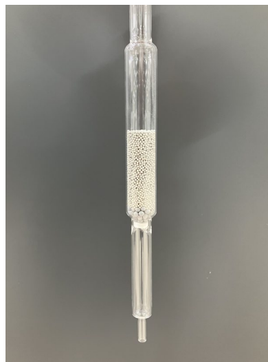
Fig. 2 Combustion Tube for High Salt Samples
