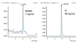
Figure 2 XICs of NDMA of 1 ng/mL and IS (NDMA-d6) of 40 ng/mL.
