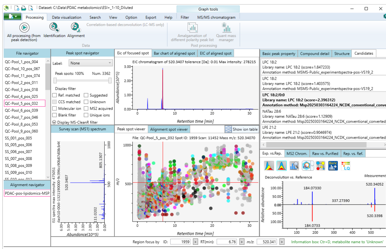
Fig. 2 MS-DIAL was used to process LabSolutions raw data files to find features that behaved as chromatographic components and align individual components as features across samples. Once all features are aligned across all samples, statistical analysis is applied to identify features that are differentially expressed between the control and treatment groups.
