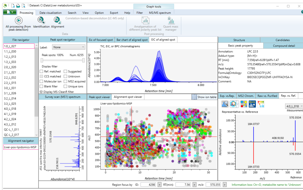
Fig. 2 MS-DIAL was used to process LabSolutions raw data files to find and align features that behaved as chromatographic peaks. The lipidomics workflow was applied in MS-DIAL enabling annotation of lipids to the 'in-silico retention time- and MS/MS database for LC/MS/MS based lipidomics'.
