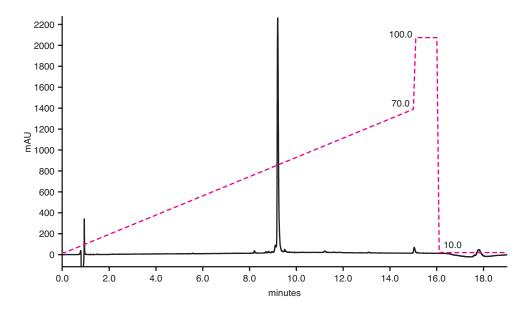
Figure 2: Campath FAb analysis on an Accucore 150-C4 HPLC column
