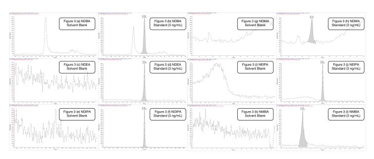
Figure 3. Chromatogram of solvent blank and standard at 0.03 ppm with regard to API sample concentration for NDBA (a-b), NDEA (c-d), NDIPA (e-f), NDMA (g-h), NEIPA (i-j), and NMBA (k-l).
