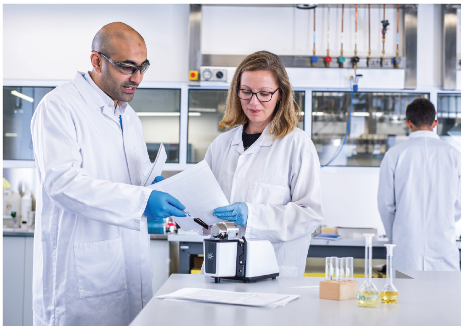
Figure 1. The benchtop Agilent Cary 630 FTIR spectrometer is versatile, innovative, and intuitive, providing quantitative and qualitative information for the analysis of solids, liquids, and gases.
