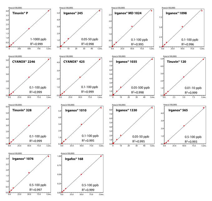
Fig. 6 Calibration Curves of 14 Polymer Additive Components
