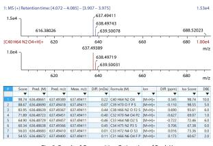
Fig. 2 Result of Composition Estimation of Peak X (Top: Measured Spectrum, Middle: Theoretical Spectrum, Bottom: Candidates of Compositional Formula)
