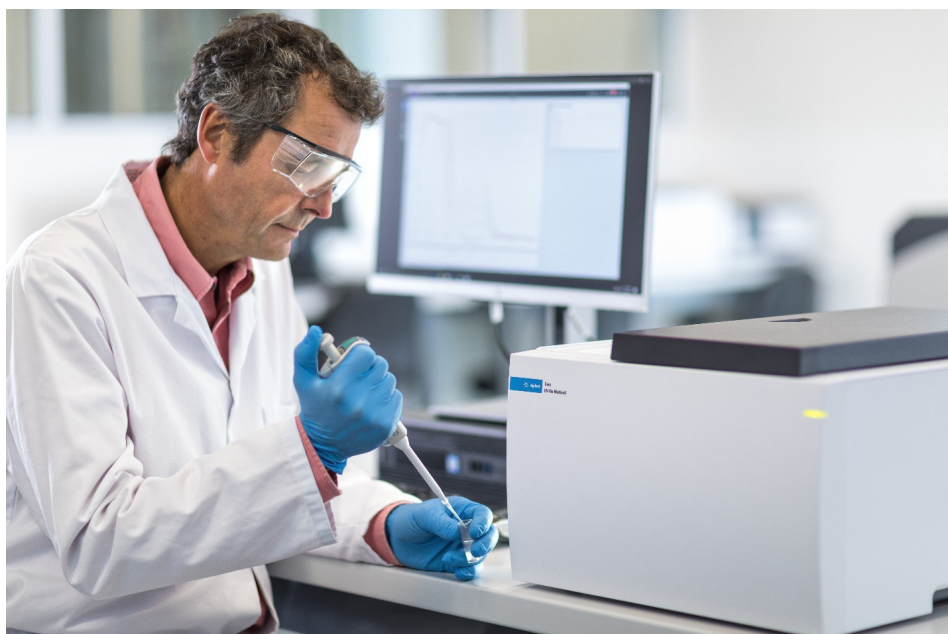
Figure 2. The Agilent Cary 3500 UV-Vis multicell spectrophotometer can be used for up to four temperature experiments, across eight cuvette positions, simultaneously.
