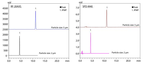
Fig. 1 Chromatograms of IPMP Standard Solution (5 mg/L)
