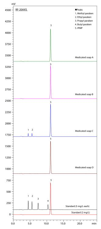
Fig. 6 Chromatograms of Medicated Soaps (Particle size 5 µm column, RF-20AXS)
