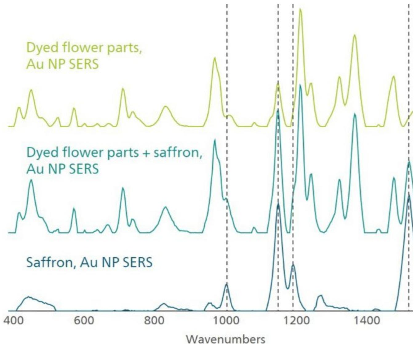
**Figure 2.** Visual confirmation in the SERS spectra of Sudan 1 (top), Saffron (bottom), and an experimental mixture of both.
