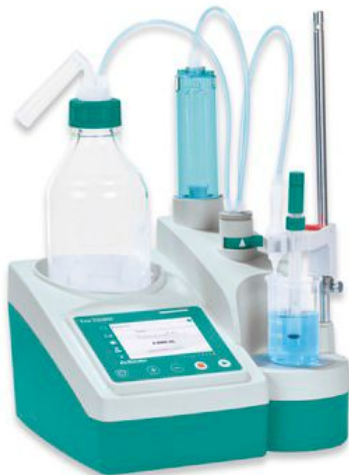
Figure 1. Eco Titrator used for the analysis of sulfur dioxide in TCM products.
