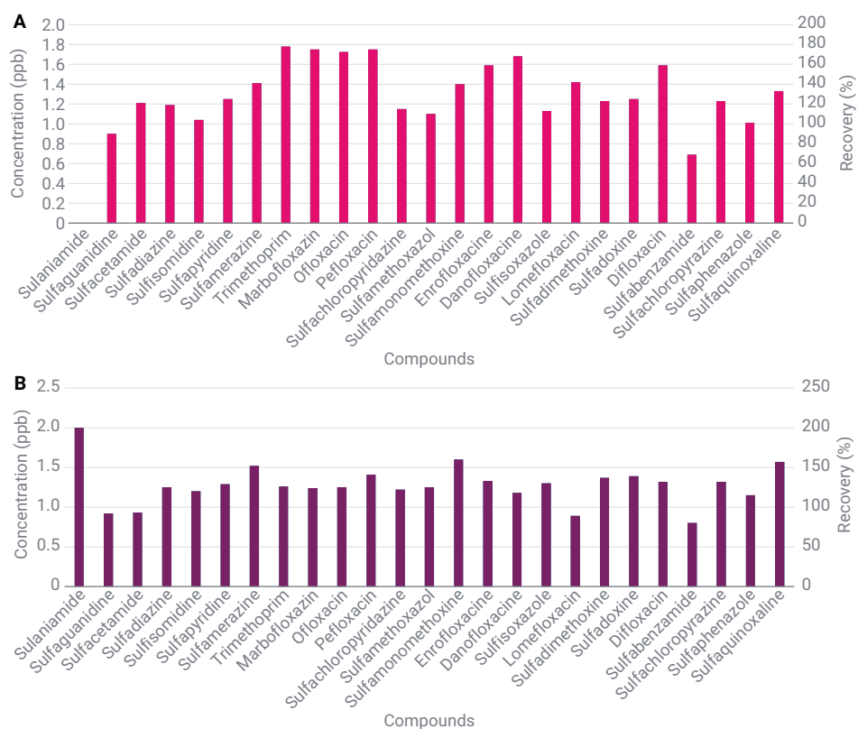
Figure 5. (A) Quantified concentration and recovery percentage of a 1 ppb spiked meat sample using pure solvent calibration. (B) Quantified concentration and recovery percentage of the 1 ppb sample measured with the matrix-matched calibration.
