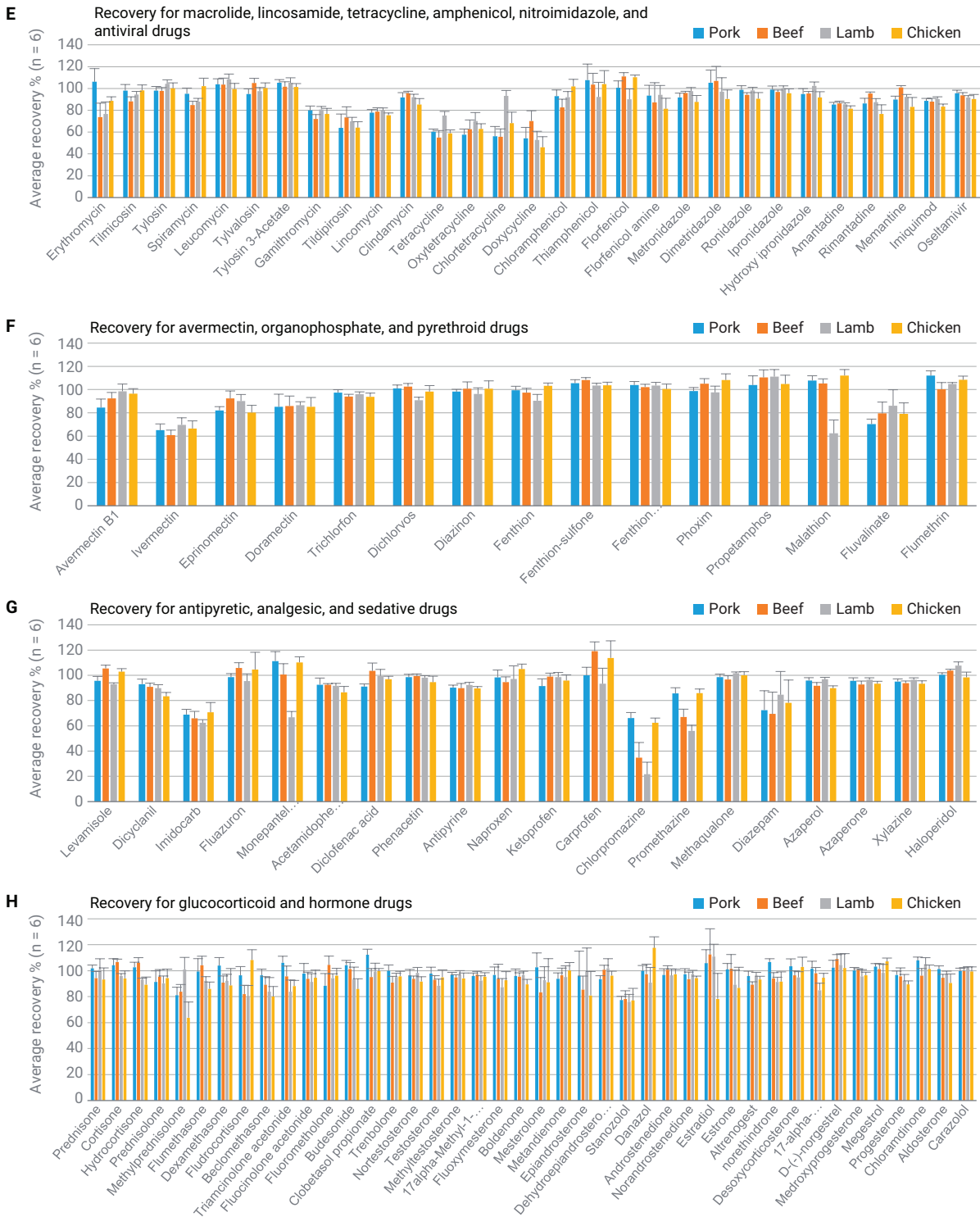
Figure 2. Recoveries of 193 veterinary drugs in pork, beef, lamb, and chicken. The sample spiking level was 5 µg/kg.
