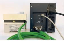
✓ Verify the location of the green serial cable from the Peltier controller to the Domino™. It mustn't be on the working area of Andrew.
