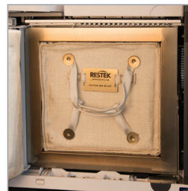
Figure 5: A correctly installed plate insert should be flush with the edge of the oven.
