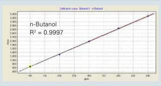
The calibration curves shown above clearly indicate that the system is well suited for the analysis of the different solvent types.
