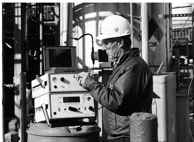
Figure A. MTI Trapper 2000 Concentrator and P200 Micro Gas Chromatograph
