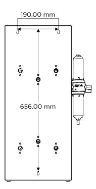
The generator can be wall mounted, **If do not wish to wall mount your generator** proceed to step 4.
