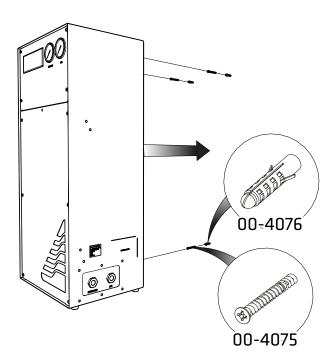
With the holes drilled in your desired location, fit the  $3 \times 10$  No. 8 Screw 00-4075 to the wall and mount your generator onto them.
