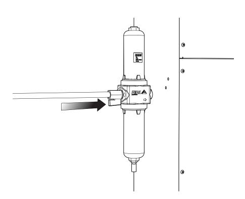
Attach your house air supply to the **BA filter** at the **left side** of the generator. Ensure the valve on the filter is at the **open** position.
