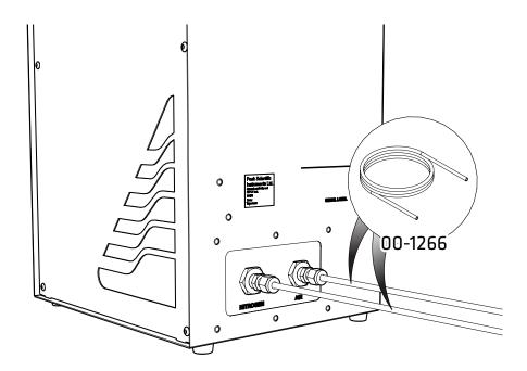
Attach the supplied 1/4" Teflon Tubing 00-1266 and connect this to the two 1/4" x 1/4" Compression Fittings 02-4421.
