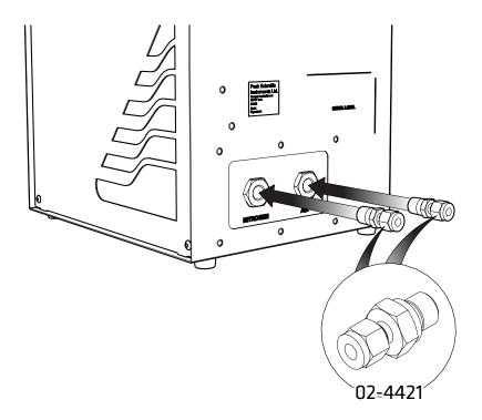
Select the 1/4" x 1/4" Compression Fittings 02-4421 and attach them to the Nitrogen and Air outlets at the right side of the generator. It is recommended that PTFE tape is applied to the threads to ensure a leak-tight fit.
