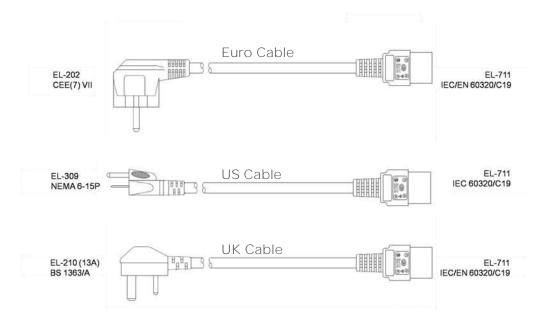
For cables pertaining to countries not displayed above, it is the responsibility of the end user to provide an appropriate power cable which meets the requirements defined in the Technical Specification section on page 6.
