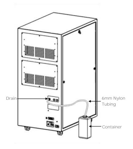
Connect the 2m Nylon tube to the drain outlet, ensure the tube is pushed fully in and gripped securely by the fitting.
