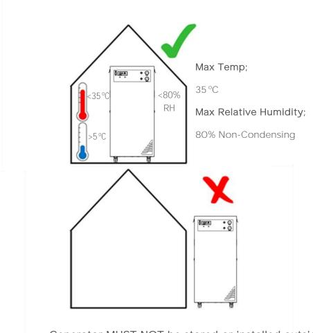
Generator MUST NOT be stored or installed outside.
