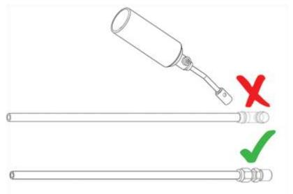
Soldering may lead to contamination. Compression fittings recommended.
