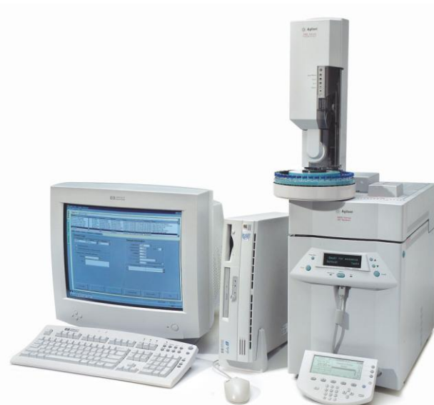
Figure 1-1. Sherlock Microbial Identification System with Agilent 6850 Series gas chromatograph.
