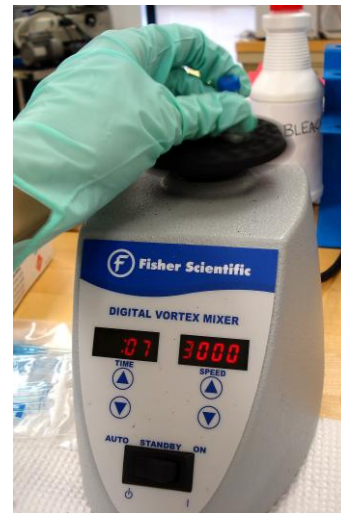
Figure 2-7. Vortexing steps. The vortexer is used after the addition of Reagent 1 for 10 seconds and again after Reagent 2 for 3 seconds.
