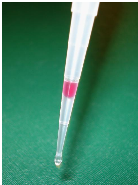
Figure 2-10. Erroneous Sample extract containing aqueous layer. If the pipette contains red dye, it contains some of the aqueous layer. The last step should be redone. The aqueous layer will degrade the inlet and potentially damage the column.
